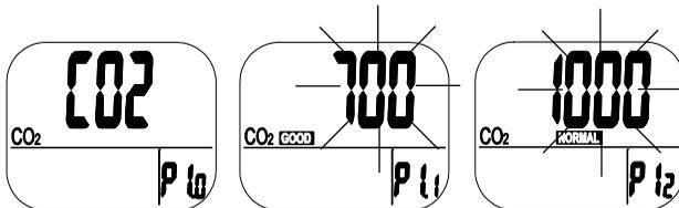
Press the LOG/▲ or MIN/MAX▼ button to increase or decrease the value. Each press adjusts in 100ppm increments. The alarm range is 0 to 700ppm.
